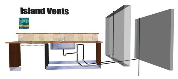
The purpose of this Information Bulletin is to ensure that **Designers** and **Installers** are aware of an **acceptable** method of venting Island Fixtures in Alberta. Any alternate configuration will require permission from the authority having jurisdiction before work proceeds (**Note: The Figure A.2.4.8.2.(1)** in **Appendix A of the NPC is not an acceptable solution).**
