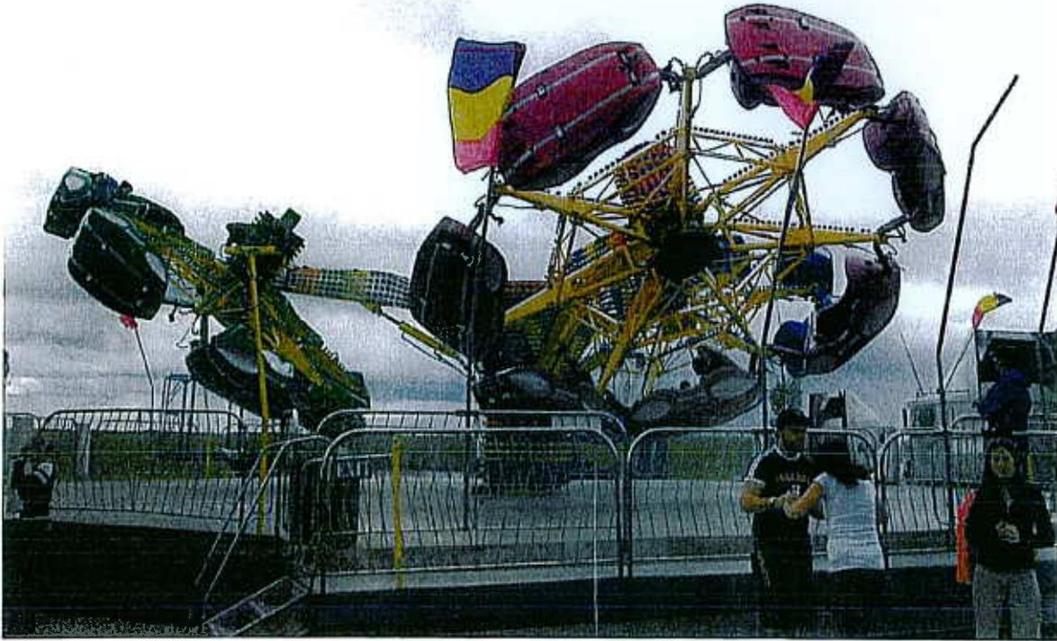
The Scorpion consists of a central column rotating at 10 rpm to which three sweep arms are attached. At the ends of the sweeps are secondary spinner sweeps rotating in the opposite sense at 33 rpm. The cars are suspended front and rear and are allowed to swing freely. The main sweep arms raise and tilt as can be seen in the photo above.
